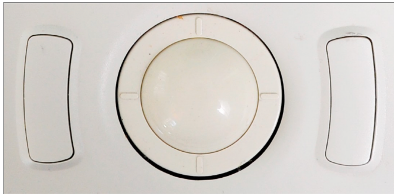
Figure 30: Click freeze and scroll with the trackball to “cineloop back” to the optimal image for taking a measurement.
